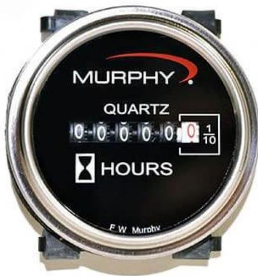
The TM Series hourmeters record the operating time of vehicles or powered equipment. They are electromechanical and have a quartz base time counter that insures accuracy (better than  $\pm 0.02\%$  over the entire range). They can record up to 99,999.9 hours (9,999.9 for TM612/624) and include an automatic recycle to zero hours feature.
