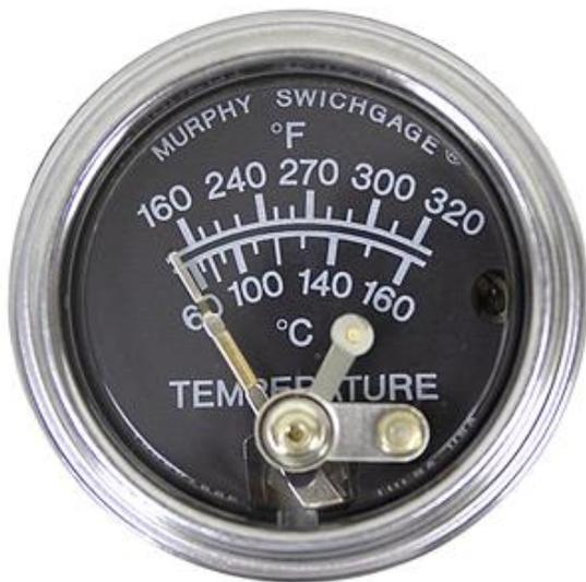
New MURPHY Switchgauge model 10-35-0949 fluid temperature gauge with high limit switch. Can be used with coolant, oil, diesel fuel or hydraulic fluid. 1/16" Hex wrench adjustment knob on front to adjust switch set point
