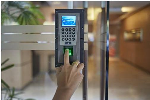
An access control point, which can be a door, turnstile, parking gate, elevator, or other physical barrier, where granting access can be electronically controlled. Typically, the access point is a door. An electronic access control can contain several elements.
