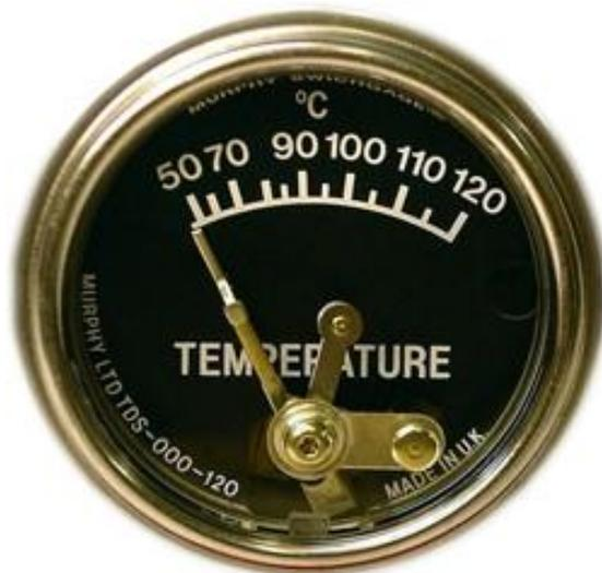
The 20 Series (2 inch/51 mm dial) and the 25 Series (2-1/2 inch/64 mm dial) Switchgauge models are diaphragm-actuated, temperature-indicating gages with built-in electrical switches for tripping alarms and/or shut-down devices.
